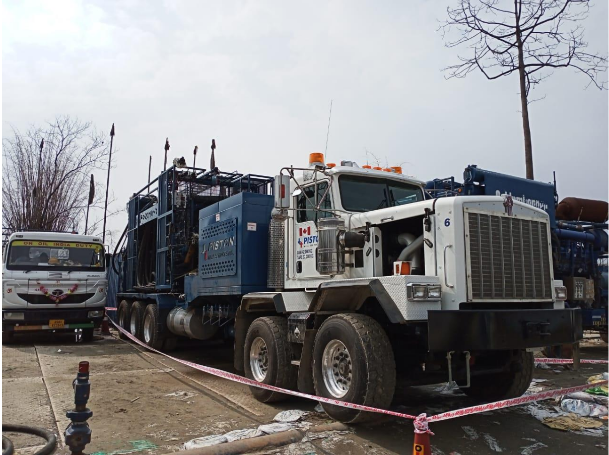
The snubbing unit which has been brought from Calgary, Canada reached Baghjan well site yesterday evening
